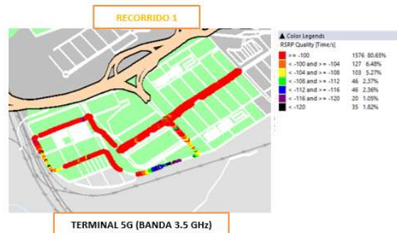
Figure 25. GHz RSRP Quality Route1 based on Site Survey measurements
