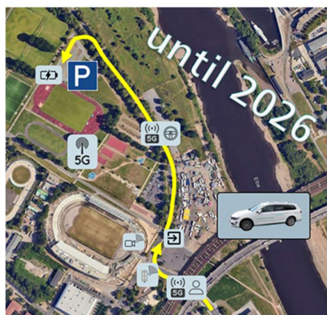
Figure 56. 5G remote automated driving route
